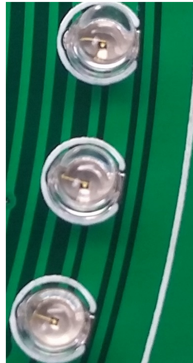
Figure 22 – Internal wires point the same way
