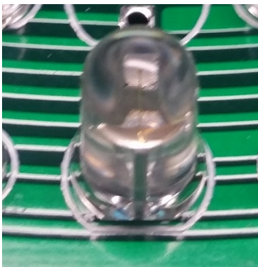
Figure 23 5mm LED flat spot
