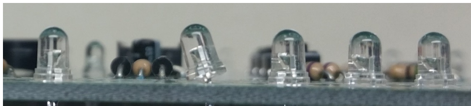
Figure 30 - LED not snug against board, needs rework
