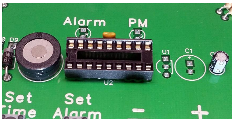
Figure 19 – BZ1 and C2 installed – note their orientation
