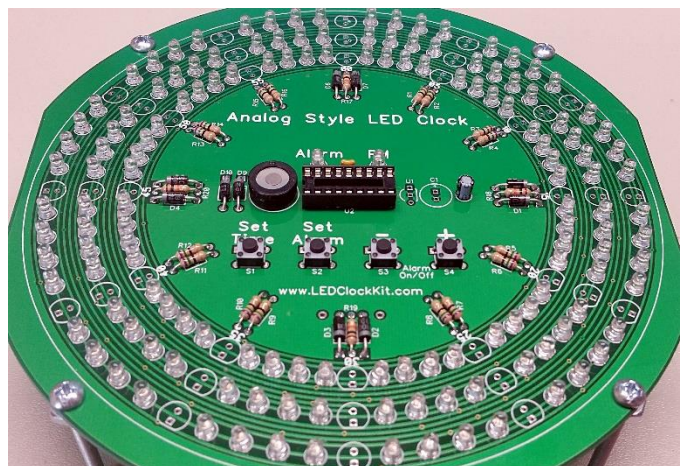
Figure 29 – All 3mm Yellow LEDs installed
